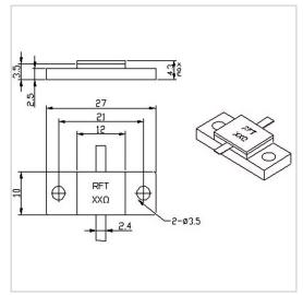
RF Solution offer a wide selection of Flanged Resistor for global customers. RFTXX-300RM2710 is a Flanged Resistor in Capacitance of 5.0 PF@100 $\Omega$ . It is made of high quality materials under a high standard, the Resistance of this product is XX  $\Omega$  (10~1000 $\Omega$  Customizable), Resistance Tolerance is  $\pm 5\%$  and Temperature Coefficient Max is 150 ppm/°C. The component has a good working performance and stability, it is ideal for handling a Power of 300 W.
