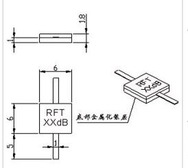
RF Solution offer a wide selection of Leaded Attenuator for global customers. RFTXX-30AM0606-6 is a Leaded Attenuator in Frequency Range of DC~6.0 GHz. It is made of high quality materials under a high standard, the Attenuation Value of this product is ①01-10 dB②15,20 dB③25,30 dB, Attenuation Tolerance is ①±0.6 dB②±0.8 dB③±1.0 dB and VSWR Max is 1.25. The component has a good working performance and stability, it is ideal for handling a Rated Power of 30 W.
