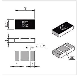
RF Solution offer a wide selection of Chip Resistor for global customers. RFTXX-30CR2550C is a Chip Resistor in Resistance Range of XX  $\Omega$  ( $10\sim3000\Omega$  Customizable). It is made of high quality materials under a high standard, the Resistance Tolerance of this product is  $\pm5\%$ , Substrate Material is BeO and Resistive Element is Thick Film. The component has a good working performance and stability, it is ideal for handling a Power of 30 W.
