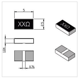
RF Solution offer a wide selection of Chip Resistor for global customers. RFTXX-30CR2550TA is a Chip Resistor in Resistance Range of XX  $\Omega$  ( $10\sim3000\Omega$  Customizable). It is made of high quality materials under a high standard, the Resistance Tolerance of this product is  $\pm5\%$ , Substrate Material is BeO and Resistive Element is Thick Film. The component has a good working performance and stability, it is ideal for handling a Power of 30 W.
