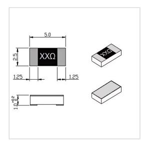
RF Solution offer a wide selection of Chip Resistor for global customers. RFTXX-30CR2550W is a Chip Resistor in Resistance Range of XX  $\Omega$  ( $10\sim3000\Omega$  Customizable). It is made of high quality materials under a high standard, the Resistance Tolerance of this product is  $\pm5\%$ , Substrate Material is BeO and Resistive Element is Thick Film. The component has a good working performance and stability, it is ideal for handling a Power of 30 W.
