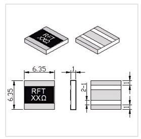
RF Solution offer a wide selection of Chip Resistor for global customers. RFTXX-30CR6363C is a Chip Resistor in Resistance Range of XX  $\Omega$  ( $10\sim3000\Omega$  Customizable). It is made of high quality materials under a high standard, the Resistance Tolerance of this product is  $\pm5\%$ , Substrate Material is BeO and Resistive Element is Thick Film. The component has a good working performance and stability, it is ideal for handling a Power of 30 W.
