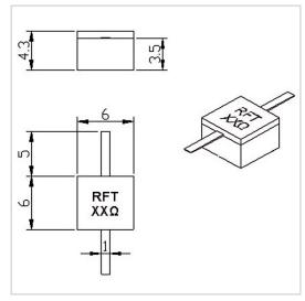
RF Solution offer a wide selection of Leaded Resistor for global customers. RFTXX-30RM0606F is a Leaded Resistor in Capacitance of 1.2 PF@100 $\Omega$ . It is made of high quality materials under a high standard, the Resistance Range of this product is XX  $\Omega$  (10-3000 $\Omega$  Customizable), Resistance Tolerance is  $\pm 5\%$  and Temperature Coefficient Max is 150 ppm/°C. The component has a good working performance and stability, it is ideal for handling a Power of 30 W.
