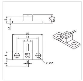
RF Solution offer a wide selection of Flanged Resistor for global customers. RFTXX-30RM2006F is a Flanged Resistor in Capacitance of 1.2 PF@100 $\Omega$ . It is made of high quality materials under a high standard, the Resistance of this product is XX  $\Omega$  (10~2000 $\Omega$  Customizable), Resistance Tolerance is  $\pm 5\%$  and Temperature Coefficient Max is 150 ppm/°C. The component has a good working performance and stability, it is ideal for handling a Power of 30 W.
