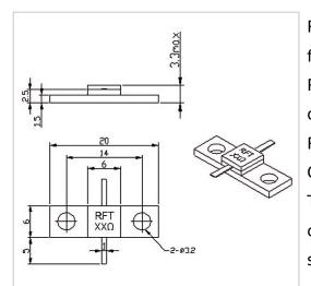
RF Solution offer a wide selection of Flanged Resistor for global customers. RFTXX-30RM2006 is a Flanged Resistor in Capacitance of 2.6 PF@100 $\Omega$ . It is made of high quality materials under a high standard, the Resistance of this product is XX  $\Omega$  (10~2000 $\Omega$ Customizable), Resistance Tolerance is ±5% and Temperature Coefficient Max is 150 ppm/°C. The component has a good working performance and stability, it is ideal for handling a Power of 30 W.
