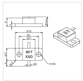
RF Solution offer a wide selection of Flanged Resistor for global customers. RFTXX-400RM2813K is a Flanged Resistor in Capacitance of 2.0 PF@100 $\Omega$ . It is made of high quality materials under a high standard, the Resistance of this product is XX  $\Omega$  (10~1000 $\Omega$  Customizable), Resistance Tolerance is  $\pm 5\%$  and Temperature Coefficient Max is 150 ppm/°C. The component has a good working performance and stability, it is ideal for handling a Power of 400 W.
