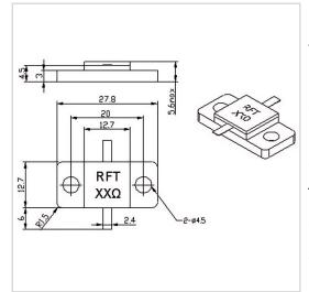
RF Solution offer a wide selection of Flanged Resistor for global customers. RFTXX-400RM2813 is a Flanged Resistor in Capacitance of 8.5 PF@100 $\Omega$ . It is made of high quality materials under a high standard, the Resistance of this product is XX  $\Omega$  (10~1000 $\Omega$ Customizable), Resistance Tolerance is ±5% and Temperature Coefficient Max is 150 ppm/°C. The component has a good working performance and stability, it is ideal for handling a Power of 400 W.
