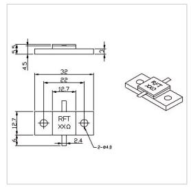
RF Solution offer a wide selection of Flanged Resistor for global customers. RFTXX-400RM3213 is a Flanged Resistor in Capacitance of 8.5 PF@100 $\Omega$ . It is made of high quality materials under a high standard, the Resistance of this product is XX  $\Omega$  (10~1000 $\Omega$  Customizable), Resistance Tolerance is  $\pm 5\%$  and Temperature Coefficient Max is 150 ppm/°C. The component has a good working performance and stability, it is ideal for handling a Power of 400 W.
