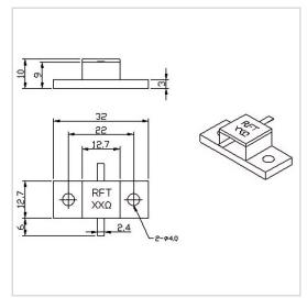
RF Solution offer a wide selection of Flanged Resistor for global customers. RFTXX-500RM3213K is a Flanged Resistor in Capacitance of 2.0 PF@100 $\Omega$ . It is made of high quality materials under a high standard, the Resistance of this product is XX  $\Omega$  (10~1000 $\Omega$  Customizable), Resistance Tolerance is  $\pm 5\%$  and Temperature Coefficient Max is 150 ppm/°C. The component has a good working performance and stability, it is ideal for handling a Power of 500 W.
