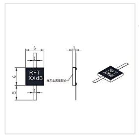
RF Solution offer a wide selection of Flanged Attenuator for global customers. RFTXX-60AJ0606-6 is a Flanged Attenuator in Frequency Range of DC~6.0 GHz. It is made of high quality materials under a high standard, the Attenuation Value of this product is 30 dB, Attenuation Tolerance is  $\pm 1.0$  dB and VSWR Max is 1.25. The component has a good working performance and stability, it is ideal for handling a Rated Power of 60 W.
