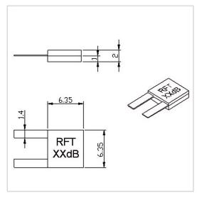
RF Solution offer a wide selection of Leaded Attenuator for global customers. RFTXX-60AM6363C-3 is a Leaded Attenuator in Frequency Range of DC~3.0 GHz. It is made of high quality materials under a high standard, the Attenuation Value of this product is 01,02,03,04,08 dB016 dB020 dB, Attenuation Tolerance is 020.6 dB020 dB, Attenuation Tolerance is 020.6 dB020 dB and VSWR Max is 1.25. The component has a good working performance and stability, it is ideal for handling a Rated Power of 60 W.
