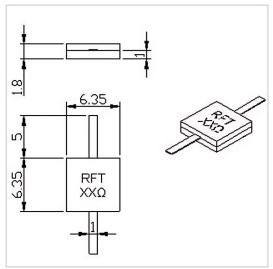
RF Solution offer a wide selection of Leaded Resistor for global customers. RFTXX-60RM6363 is a Leaded Resistor in Capacitance of /. It is made of high quality materials under a high standard, the Resistance Range of this product is XX  $\Omega$  (10-3000 $\Omega$  Customizable), Resistance Tolerance is  $\pm 5\%$  and Temperature Coefficient Max is 150 ppm/°C. The component has a good working performance and stability, it is ideal for handling a Power of 60 W.
