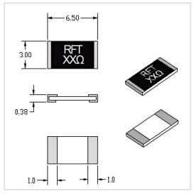
RF Solution offer a wide selection of Chip Resistor for global customers. RFTXXA-02CR3065B is a Chip Resistor in Resistance Range of XX  $\Omega$  ( $10\sim3000\Omega$  Customizable). It is made of high quality materials under a high standard, the Resistance Tolerance of this product is  $\pm5\%$ , Substrate Material is Al2O3 and Resistive Element is Thick Film. The component has a good working performance and stability, it is ideal for handling a Power of 2 W.
