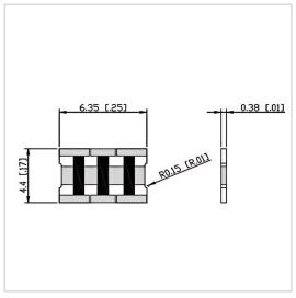
RF Solution offer a wide selection of Microstrip Attenuator for global customers. RFTXXA-02MA4463-18 is a Microstrip Attenuator in Frequency Range of DC $\sim$ 18.0 GHz. It is made of high quality materials under a high standard, the Attenuation Value of this product is 15/20/25/30 dB, Attenuation Tolerance is  $\pm$ 1.0 dB and VSWR Max is 1.30. The component has a good working performance and stability, it is ideal for handling a Rated Power of 2 W.
