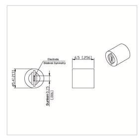
RF Solution offer a wide selection of Microstrip Attenuator with Sleeve for global customers. RFTXXA-02TA5465-18 is a Microstrip Attenuator with Sleeve in Frequency Range of DC $\sim$ 18.0GHz. It is made of high quality materials under a high standard, the Attenuation Value of this product is 12/20/25/30 dB , Attenuation Tolerance is  $\pm 1.0$  dB and VSWR Max is 1.30. The component has a good working performance and stability, it is ideal for handling a Power of 2 W.
