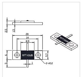
RF Solution offer a wide selection of Flanged Attenuator for global customers. RFTXXN-100AJ2006-3 is a Flanged Attenuator in Frequency Range of DC~3.0 GHz. It is made of high quality materials under a high standard, the Attenuation Value of this product is 13,20,30 dB, Attenuation Tolerance is  $\pm$ 1.0 dB and VSWR Max is 1.20. The component has a good working performance and stability, it is ideal for handling a Rated Power of 100 W.
