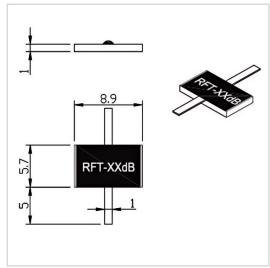
RF Solution offer a wide selection of Leaded Attenuator for global customers. RFTXXN-100AJ8957-3 is a Leaded Attenuator in Frequency Range of DC~3.0 GHz. It is made of high quality materials under a high standard, the Attenuation Value of this product is 13,20,30 dB, Attenuation Tolerance is ±1.0 dB and VSWR Max is 1.20. The component has a good working performance and stability, it is ideal for handling a Rated Power of 100 W.
