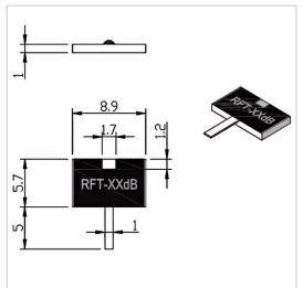
RF Solution offer a wide selection of Leaded Attenuator for global customers. RFTXXN-100AJ8957T-3 is a Leaded Attenuator in Frequency Range of DC~3.0 GHz. It is made of high quality materials under a high standard, the Attenuation Value of this product is 20,30 dB, Attenuation Tolerance is  $\pm$ 1.0 dB and VSWR Max is 1.20. The component has a good working performance and stability, it is ideal for handling a Rated Power of 100 W.
