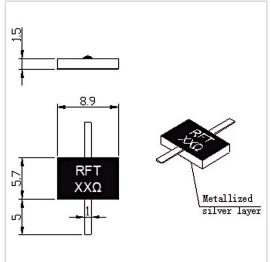
RF Solution offer a wide selection of Leaded Resistor for global customers. RFTXXN-100RJ8957B is a Leaded Resistor in Capacitance of 2.1 PF@100 $\Omega$ . It is made of high quality materials under a high standard, the Resistance Range of this product is XX  $\Omega$  (10-1500 $\Omega$  Customizable), Resistance Tolerance is  $\pm 5\%$  and Temperature Coefficient Max is 150 ppm/°C. The component has a good working performance and stability, it is ideal for handling a Power of 100 W.
