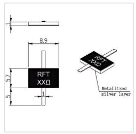
RF Solution offer a wide selection of Leaded Resistor for global customers. RFTXXN-100RJ8957 is a Leaded Resistor in Capacitance of 2.5 PF@100 $\Omega$ . It is made of high quality materials under a high standard, the Resistance Range of this product is XX  $\Omega$  (10-1500 $\Omega$  Customizable), Resistance Tolerance is  $\pm 5\%$  and Temperature Coefficient Max is 150 ppm/°C. The component has a good working performance and stability, it is ideal for handling a Power of 100 W.
