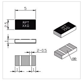
RF Solution offer a wide selection of Chip Resistor for global customers. RFTXXN-10CR2550C is a Chip Resistor in Resistance Range of XX  $\Omega$  (10~3000 $\Omega$  Customizable). It is made of high quality materials under a high standard, the Resistance Tolerance of this product is  $\pm 5\%$ , Substrate Material is AlN and Resistive Element is Thick Film. The component has a good working performance and stability, it is ideal for handling a Power of 10 W.
