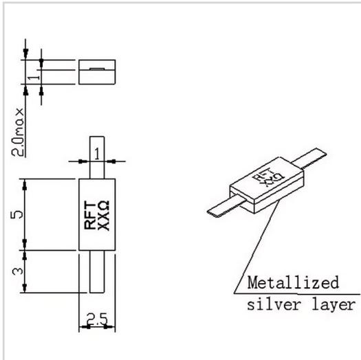
RF Solution offer a wide selection of Leaded Resistor for global customers. RFTXXN-10RM2550 is a Leaded Resistor in Capacitance of 2.4 PF@100Ω. It is made of high quality materials under a high standard, the Resistance Range of this product is XX Ω (10-3000Ω Customizable), Resistance Tolerance is ±5% and Temperature Coefficient Max is 150 ppm/°C. The component has a good working performance and stability, it is ideal for handling a Power of 5 W.
