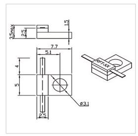
RF Solution offer a wide selection of Flanged Resistor for global customers. RFTXXN-10RM7750 is a Flanged Resistor in Capacitance of 2.4 PF@100 $\Omega$ . It is made of high quality materials under a high standard, the Resistance of this product is XX  $\Omega$  (10~3000 $\Omega$  Customizable), Resistance Tolerance is  $\pm 5\%$  and Temperature Coefficient Max is 150 ppm/°C. The component has a good working performance and stability, it is ideal for handling a Power of 10 W.
