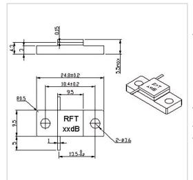
RF Solution offer a wide selection of Flanged Attenuator for global customers. RFTXXN-150AM2595B-3 is a Flanged Attenuator in Frequency Range of DC~3.0 GHz. It is made of high quality materials under a high standard, the Attenuation Value of this product is 3 dB@4 dB, Attenuation Tolerance is  $\pm 0.65 dB@\pm 0.70 dB$  and VSWR Max is 1.25. The component has a good working performance and stability, it is ideal for handling a Rated Power of 150 W.
