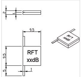
RF Solution offer a wide selection of Leaded Attenuator for global customers. RFTXXN-150AM9595B-3 is a Leaded Attenuator in Frequency Range of DC~3.0 GHz. It is made of high quality materials under a high standard, the Attenuation Value of this product is 03 dB = 04 dB, Attenuation Tolerance is  $\pm 0.65 \text{ dB} = \pm 0.7 \text{ dB}$  and VSWR Max is 1.25. The component has a good working performance and stability, it is ideal for handling a Rated Power of 150 W.
