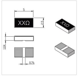
RF Solution offer a wide selection of Chip Resistor for global customers. RFTXXN-20CR2550TA is a Chip Resistor in Resistance Range of XX  $\Omega$  ( $10\sim3000\Omega$  Customizable). It is made of high quality materials under a high standard, the Resistance Tolerance of this product is  $\pm5\%$ , Substrate Material is AlN and Resistive Element is Thick Film. The component has a good working performance and stability, it is ideal for handling a Power of 20 W.
