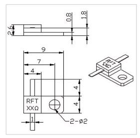
RF Solution offer a wide selection of Flanged Resistor for global customers. RFTXXN-20RM0904 is a Flanged Resistor in Capacitance of 2.3 PF@100 $\Omega$ . It is made of high quality materials under a high standard, the Resistance of this product is XX  $\Omega$  (10~3000 $\Omega$  Customizable), Resistance Tolerance is  $\pm 5\%$  and Temperature Coefficient Max is 150 ppm/°C. The component has a good working performance and stability, it is ideal for handling a Power of 10 W.
