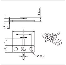
RF Solution offer a wide selection of Flanged Resistor for global customers. RFTXXN-20RM1304 is a Flanged Resistor in Capacitance of 2.3 PF@100 $\Omega$ . It is made of high quality materials under a high standard, the Resistance of this product is XX  $\Omega$  (10~3000 $\Omega$  Customizable), Resistance Tolerance is  $\pm 5\%$  and Temperature Coefficient Max is 150 ppm/°C. The component has a good working performance and stability, it is ideal for handling a Power of 20 W.
