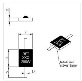
RF Solution offer a wide selection of Leaded Resistor for global customers. RFTXXN-250RJ0708 is a Leaded Resistor in Capacitance of /. It is made of high quality materials under a high standard, the Resistance Range of this product is XX  $\Omega$  (10-1000 $\Omega$  Customizable), Resistance Tolerance is  $\pm 5\%$  and Temperature Coefficient Max is 150 ppm/°C. The component has a good working performance and stability, it is ideal for handling a Power of 250 W.
