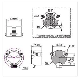
RF Solution offer a wide selection of Surface Mount Isolator for global customers. SMTG-D10 is a Surface Mount Isolator in Frequency Range of  $2.0\sim6.0$  GHz. It is made of high quality materials under a high standard, the Bandwidth Max of this product is 15%, Insertion Loss Max is  $0.30\sim0.40$  dB and Isolation Min is  $20.0\sim21.0$  dB. The component has a good working performance and stability, it is ideal for handling a Forward Power of 30 W.
