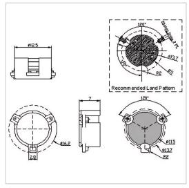
RF Solution offer a wide selection of Surface Mount Isolator for global customers. SMTG-D12.5 is a Surface Mount Isolator in Frequency Range of 700~6000 MHz. It is made of high quality materials under a high standard, the Bandwidth Max of this product is 15%, Insertion Loss Max is 0.30~0.60 dB and Isolation Min is 18.0~23.0 dB. The component has a good working performance and stability, it is ideal for handling a Forward Power of 30 W.
