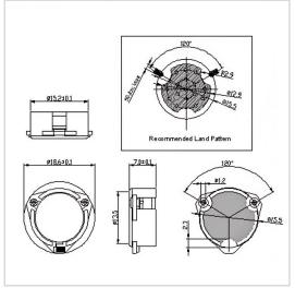
RF Solution offer a wide selection of Surface Mount Isolator for global customers. SMTG-D15 is a Surface Mount Isolator in Frequency Range of 1.0~5.0 GHz. It is made of high quality materials under a high standard, the Bandwidth Max of this product is 15%, Insertion Loss Max is 0.25~0.50 dB and Isolation Min is 20.0~25.0 dB. The component has a good working performance and stability, it is ideal for handling a Forward Power of 60 W.
