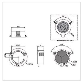
RF Solution offer a wide selection of Surface Mount Isolator for global customers. SMTG-D18 is a Surface Mount Isolator in Frequency Range of 900~2600 MHz. It is made of high quality materials under a high standard, the Bandwidth Max of this product is 5%, Insertion Loss Max is 0.25~0.50 dB and Isolation Min is 18.0~23.0 dB. The component has a good working performance and stability, it is ideal for handling a Forward Power of 100 W.
