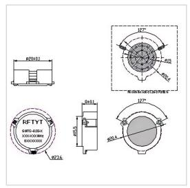
RF Solution offer a wide selection of Surface Mount Isolator for global customers. SMTG-D20 is a Surface Mount Isolator in Frequency Range of  $700\sim3000$  MHz. It is made of high quality materials under a high standard, the Bandwidth Max of this product is 20%, Insertion Loss Max is  $0.30\sim0.60$  dB and Isolation Min is  $17.0\sim23.0$  dB. The component has a good working performance and stability, it is ideal for handling a Forward Power of 60/100 W.
