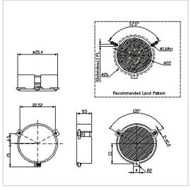
RF Solution offer a wide selection of Surface Mount Isolator for global customers. SMTG-D25.4 is a Surface Mount Isolator in Frequency Range of 400~1800 MHz. It is made of high quality materials under a high standard, the Bandwidth Max of this product is 10%, Insertion Loss Max is 0.20~0.60 dB and Isolation Min is 18.0~25.0 dB. The component has a good working performance and stability, it is ideal for handling a Forward Power of 100/200/300 W.
