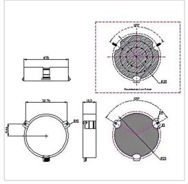
RF Solution offer a wide selection of Surface Mount Isolator for global customers. SMTG-D35 is a Surface Mount Isolator in Frequency Range of 300~600 MHz. It is made of high quality materials under a high standard, the Bandwidth Max of this product is 10%, Insertion Loss Max is 0.25~0.60 dB and Isolation Min is 18.0~25.0 dB. The component has a good working performance and stability, it is ideal for handling a Forward Power of 150 W.
