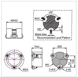
RF Solution offer a wide selection of Surface Mount Circulator for global customers. SMTH-D10 is a Surface Mount Circulator in Frequency Range of 3000~6000 MHz. It is made of high quality materials under a high standard, the Bandwidth Max of this product is 10%, Insertion Loss Max is 0.30~0.40 dB and Isolation Min is 20.0~23.0 dB. The component has a good working performance and stability, it is ideal for handling a Power of 30 W.
