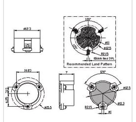
RF Solution offer a wide selection of Surface Mount Circulator for global customers. SMTH-D12.3A is a Surface Mount Circulator in Frequency Range of 1400~6000 MHz. It is made of high quality materials under a high standard, the Bandwidth Max of this product is 20%, Insertion Loss Max is 0.35~0.50 dB and Isolation Min is 18.0~23.0 dB. The component has a good working performance and stability, it is ideal for handling a Power of 30 W.
