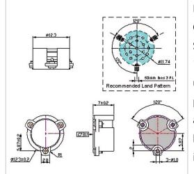
RF Solution offer a wide selection of Surface Mount Circulator for global customers. SMTH-D12.3B is a Surface Mount Circulator in Frequency Range of 1400~6000 MHz. It is made of high quality materials under a high standard, the Bandwidth Max of this product is 20%, Insertion Loss Max is 0.30~0.60 dB and Isolation Min is 17.0~23.0 dB. The component has a good working performance and stability, it is ideal for handling a Power of 30 W.
