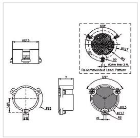
RF Solution offer a wide selection of Surface Mount Circulator for global customers. SMTH-D12.5 is a Surface Mount Circulator in Frequency Range of 800~5900 MHz. It is made of high quality materials under a high standard, the Bandwidth Max of this product is 15%, Insertion Loss Max is 0.30~0.60 dB and Isolation Min is 18.0~23.0 dB. The component has a good working performance and stability, it is ideal for handling a Power of 30/50/60/100 W.
