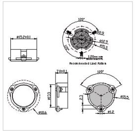
RF Solution offer a wide selection of Surface Mount Circulator for global customers. SMTH-D15 is a Surface Mount Circulator in Frequency Range of 1000~5000 MHz. It is made of high quality materials under a high standard, the Bandwidth Max of this product is 5%, Insertion Loss Max is 0.25~0.40 dB and Isolation Min is 20.0~25.0 dB. The component has a good working performance and stability, it is ideal for handling a Power of 60 W.
