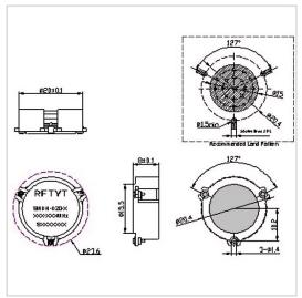
RF Solution offer a wide selection of Surface Mount Circulator for global customers. SMTH-D20 is a Surface Mount Circulator in Frequency Range of 750~2500 MHz. It is made of high quality materials under a high standard, the Bandwidth Max of this product is 20%, Insertion Loss Max is 0.30~0.60 dB and Isolation Min is 17.0~23.0 dB. The component has a good working performance and stability, it is ideal for handling a Power of 60/100 W.
