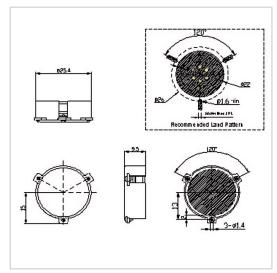
RF Solution offer a wide selection of Surface Mount Circulator for global customers. SMTH-D25.4 is a Surface Mount Circulator in Frequency Range of 400~1800 MHz. It is made of high quality materials under a high standard, the Bandwidth Max of this product is 10%, Insertion Loss Max is 0.20~0.60 dB and Isolation Min is 16.0~25.0 dB. The component has a good working performance and stability, it is ideal for handling a Power of 100/200 W.
