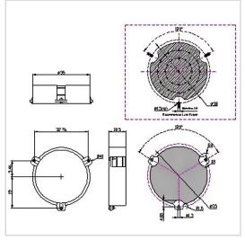
RF Solution offer a wide selection of Surface Mount Circulator for global customers. SMTH-D35 is a Surface Mount Circulator in Frequency Range of 300~1000 MHz. It is made of high quality materials under a high standard, the Bandwidth Max of this product is 10%, Insertion Loss Max is 0.30~0.80 dB and Isolation Min is 16.0~25.0 dB. The component has a good working performance and stability, it is ideal for handling a Power of 300 W.
