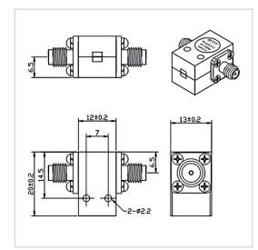
RF Solution offer a wide selection of Coaxial Isolator for global customers. TG1220CS is a Coaxial Isolator in Frequency Range of 9.0~18.0 GHz. It is made of high quality materials under a high standard, the Bandwidth Max of this product is 20%, Insertion Loss Max is 0.30~0.60 dB and Isolation Min is 18.0~23.0 dB. The component has a good working performance and stability, it is ideal for handling a Forward Power of 30 W.
