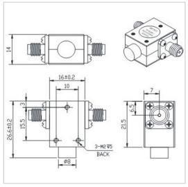
RF Solution offer a wide selection of Coaxial Isolator for global customers. TG1622BS is a Coaxial Isolator in Frequency Range of 6.0~18.0 GHz. It is made of high quality materials under a high standard, the Bandwidth Max of this product is 100%, Insertion Loss Max is 0.50~1.50 dB and Isolation Min is 9.5~20.0 dB. The component has a good working performance and stability, it is ideal for handling a Forward Power of 30 W.
